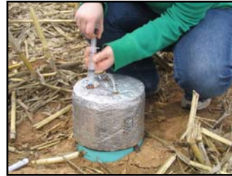
Extracting a GHG sample; injection into an vial.
