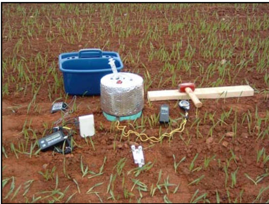
A typical GHG flux monitoring kit.
