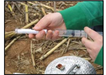
Extracting a GHG sample; injection into an vial.
